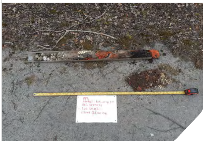
Photo 05: Core sample from WS01
