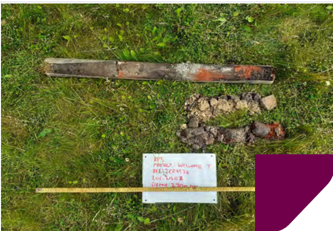
Photo 06: Core sample from WS08
