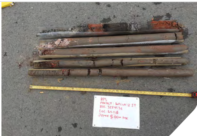
Photo 06: Core samples from WS04
