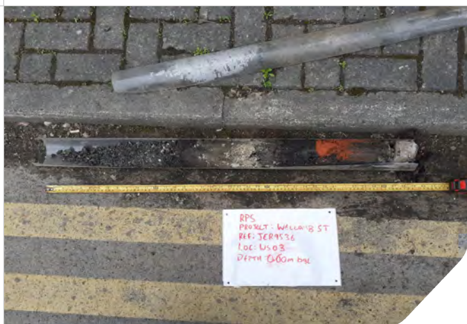
Photo 07: Core sample from WS03
