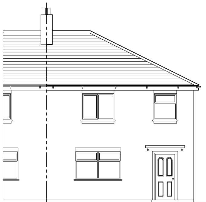
Existing Front Elevation
