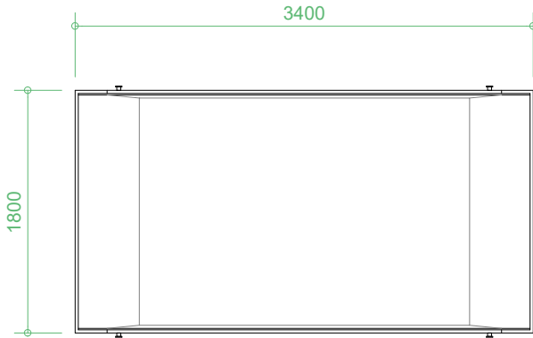
Construction Bin Plan Scale 1:50
