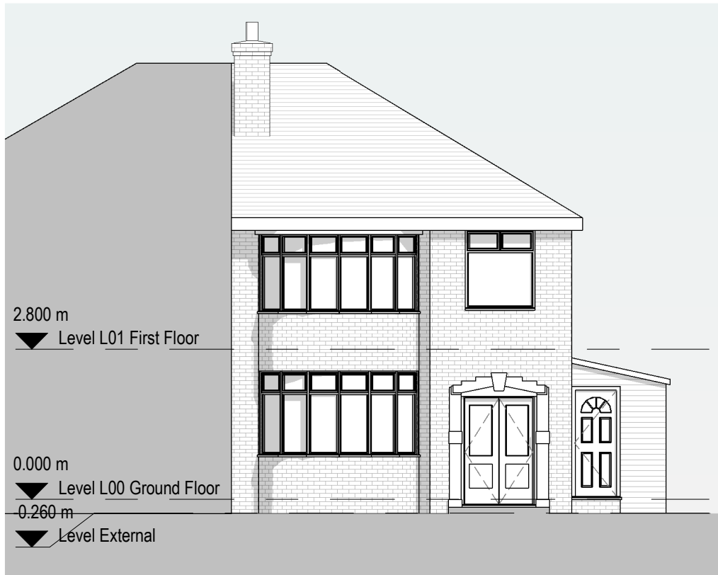
1 Existing South Elevation 1 : 100
