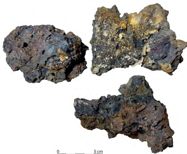
Plate 2: vitrified coal ash or clinker found the fill of French drain [05] in Trial Pit 3.
