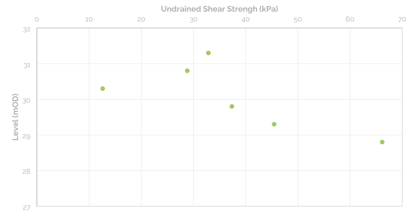
Plate 7. Undrained Shear Strength versus Level (mOD) for Made Ground
