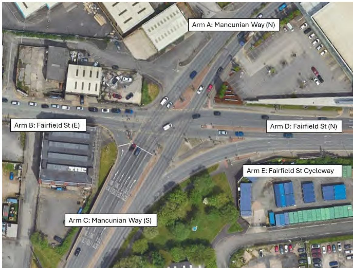
Figure 15: Existing Mancunian Way/Fairfield St junction layout
