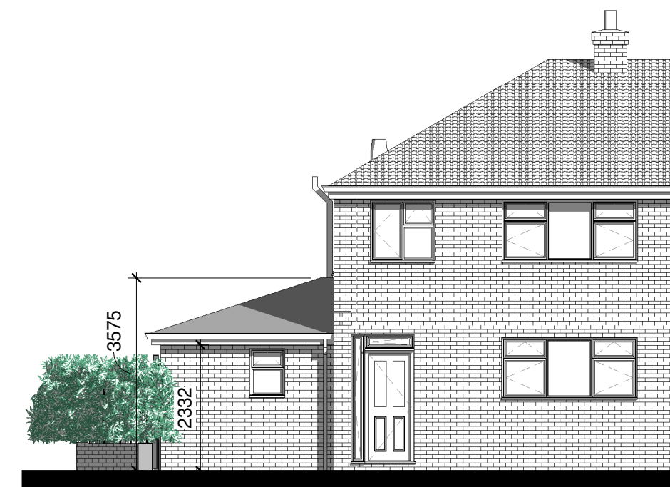
Proposed Part Front Elevation
