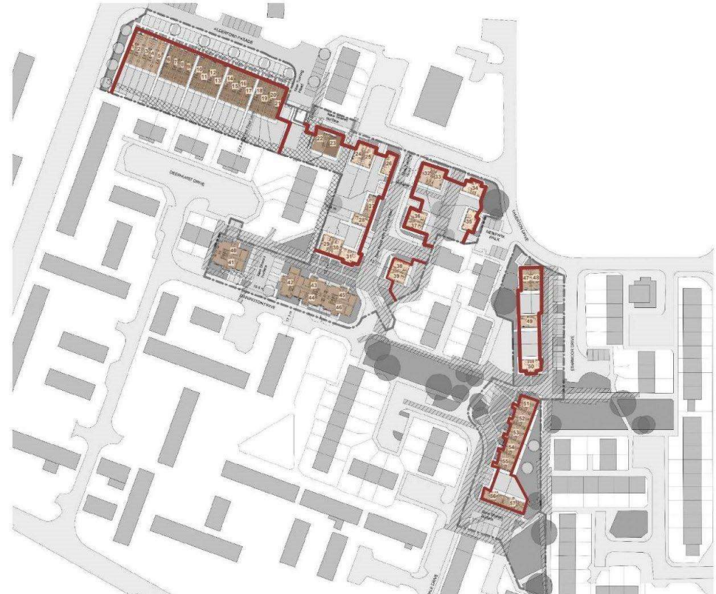
Site plan showing proposed development 'clusters' linked by boundary walls
