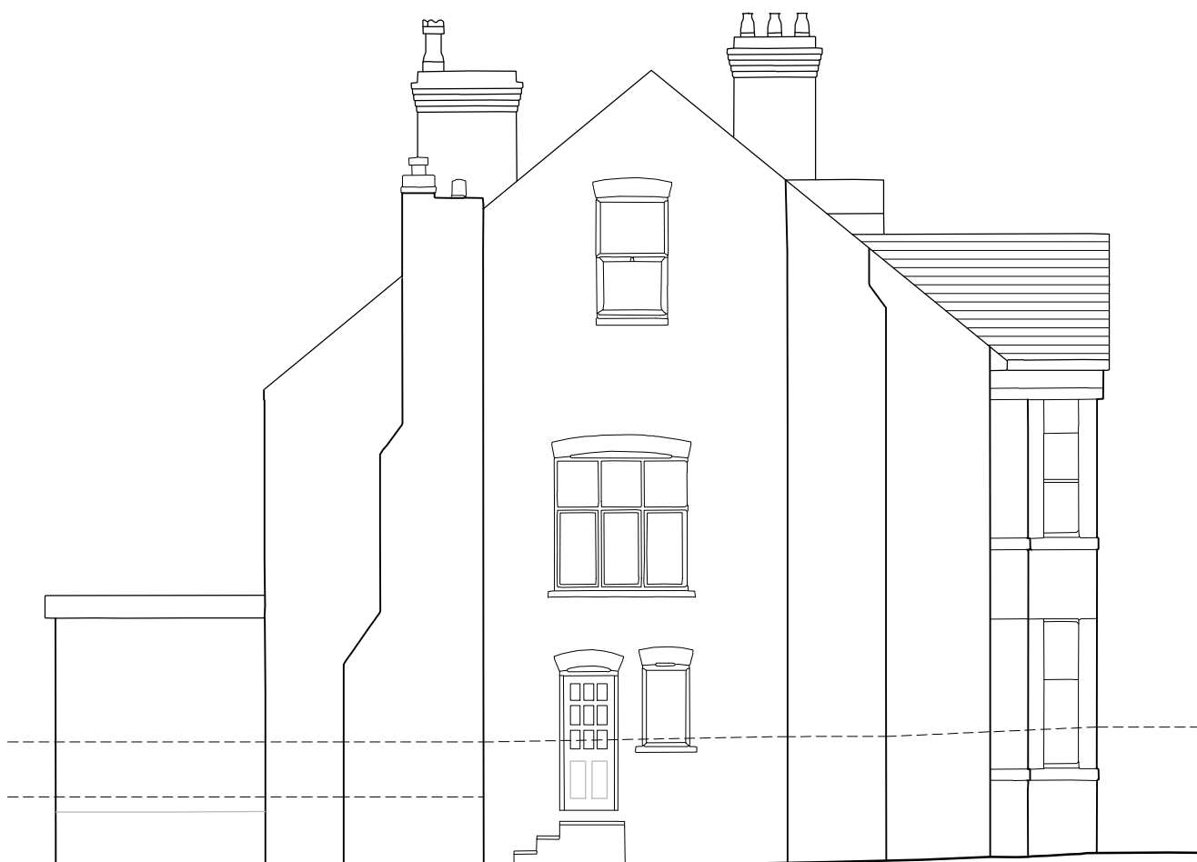
Existing North Elevation Scale 1:100@A3
