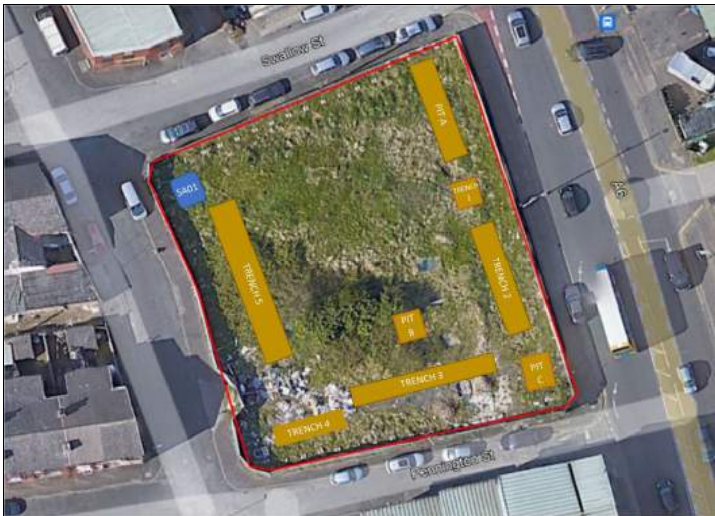
Figure 8: Exploratory Hole Location Plan (Trenching SI)
