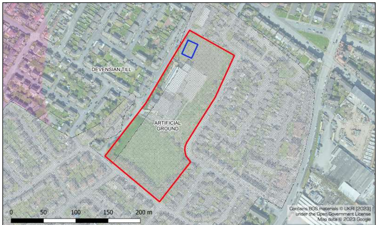
Figure 2-I: Extract from BGS showing superficial geology at the site
