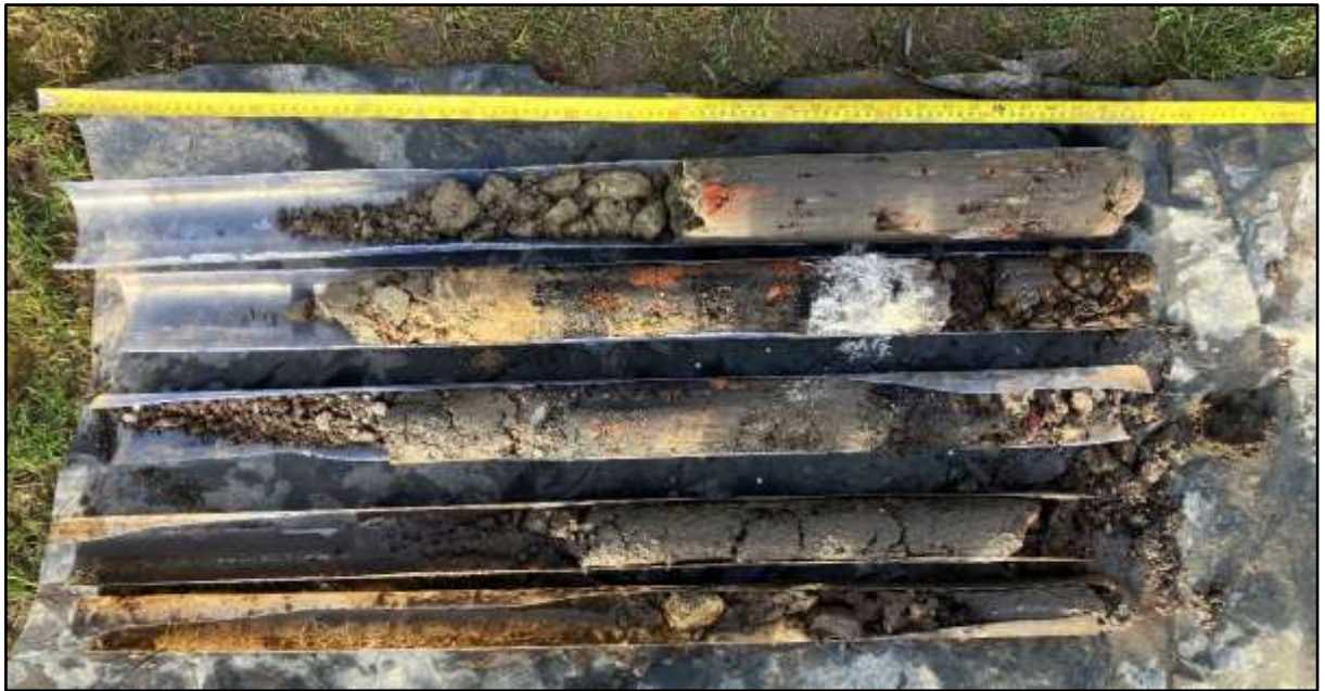
Figure 5-A: Made Ground encountered in WS01
