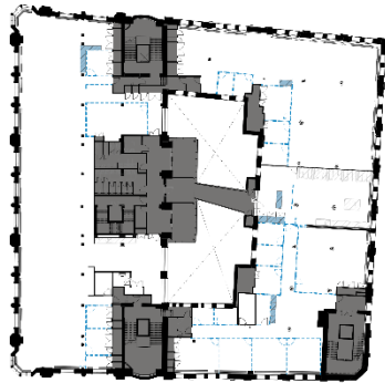
Existing partitions to be stripped-out indicated in blue
