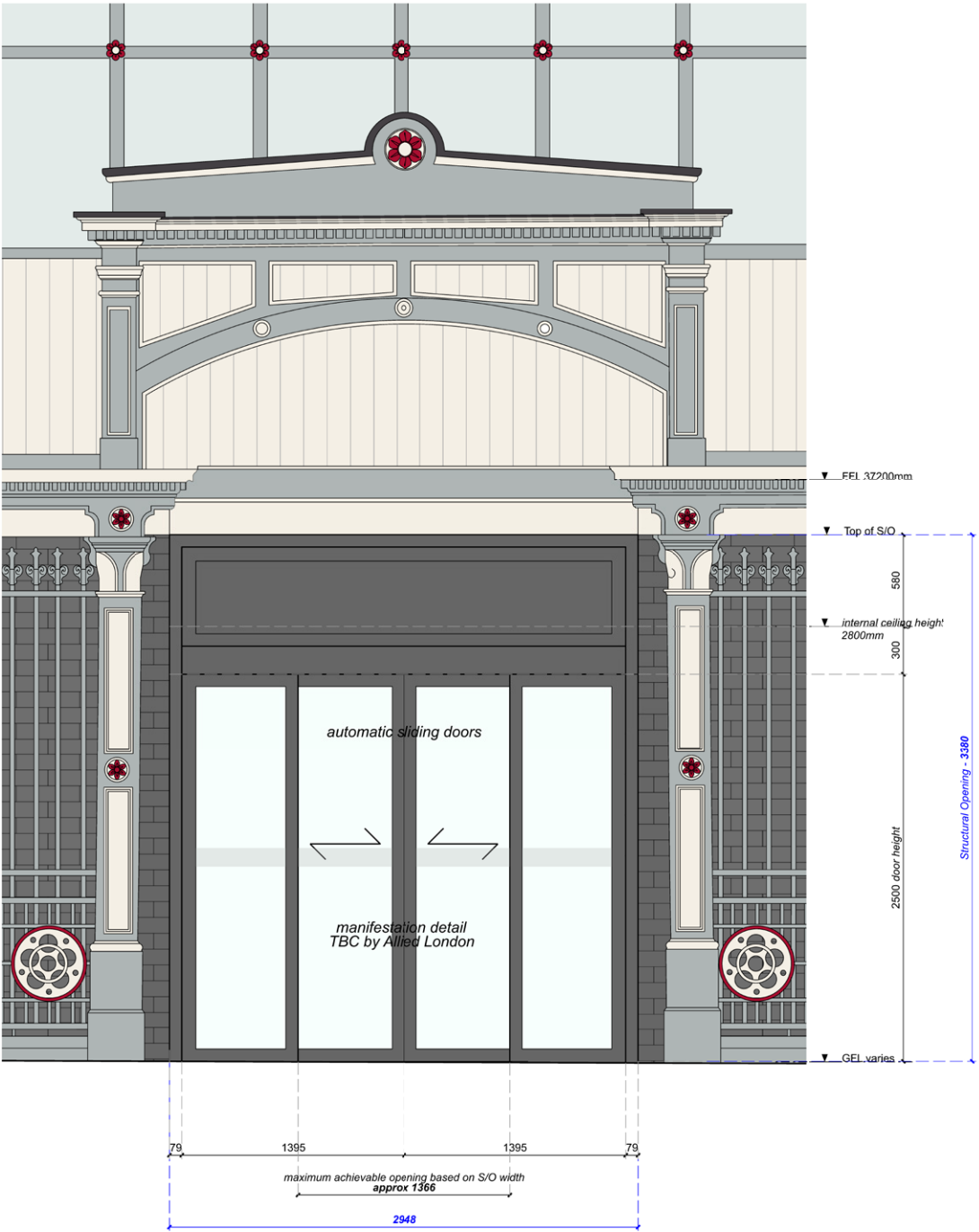
Lower Byrom Street Proposed Automatic Doors Refurbished Doors Open
