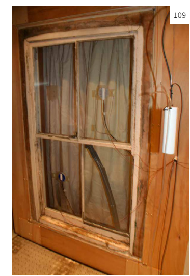
Image 109 Testing windows in the climate chamber at Glasgow Caledonian University.
