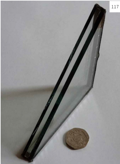
Image 117 This slim profile IGU comprises 3mm outer glazing a 3mm gas filled cavity and 4mm Low-E inner glazing giving a total thickness of 10mm.
