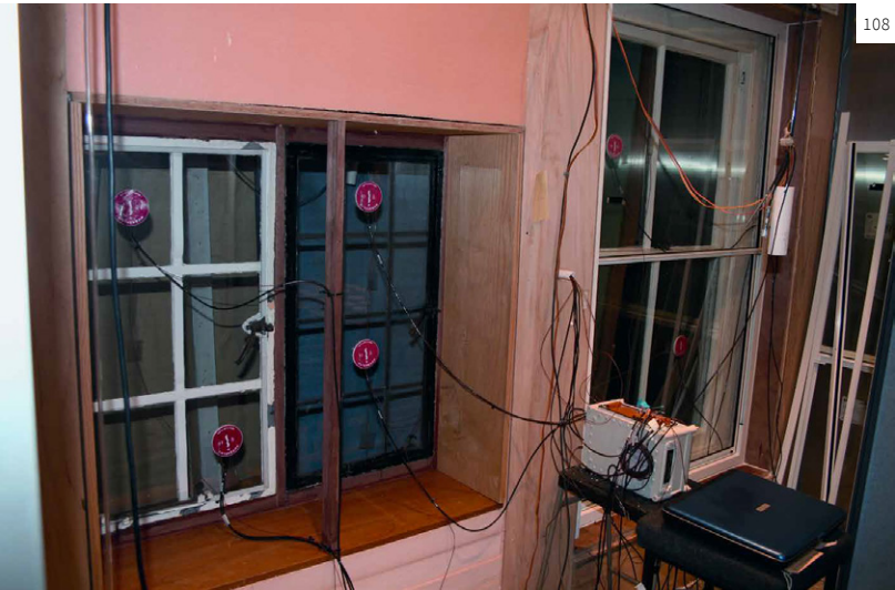
Image 108 Testing windows in the climate chamber at Glasgow Caledonian University.
