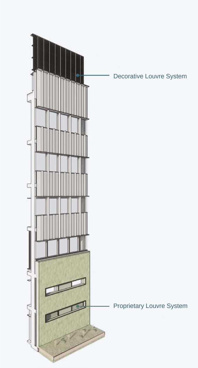
Bespoke perforated metal cladding, functioning to allow ventilation to the open top plant areas both at roof level and annexe
