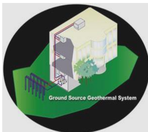
Fig. 5.1 – Ground-Source Heat Pump Installation
