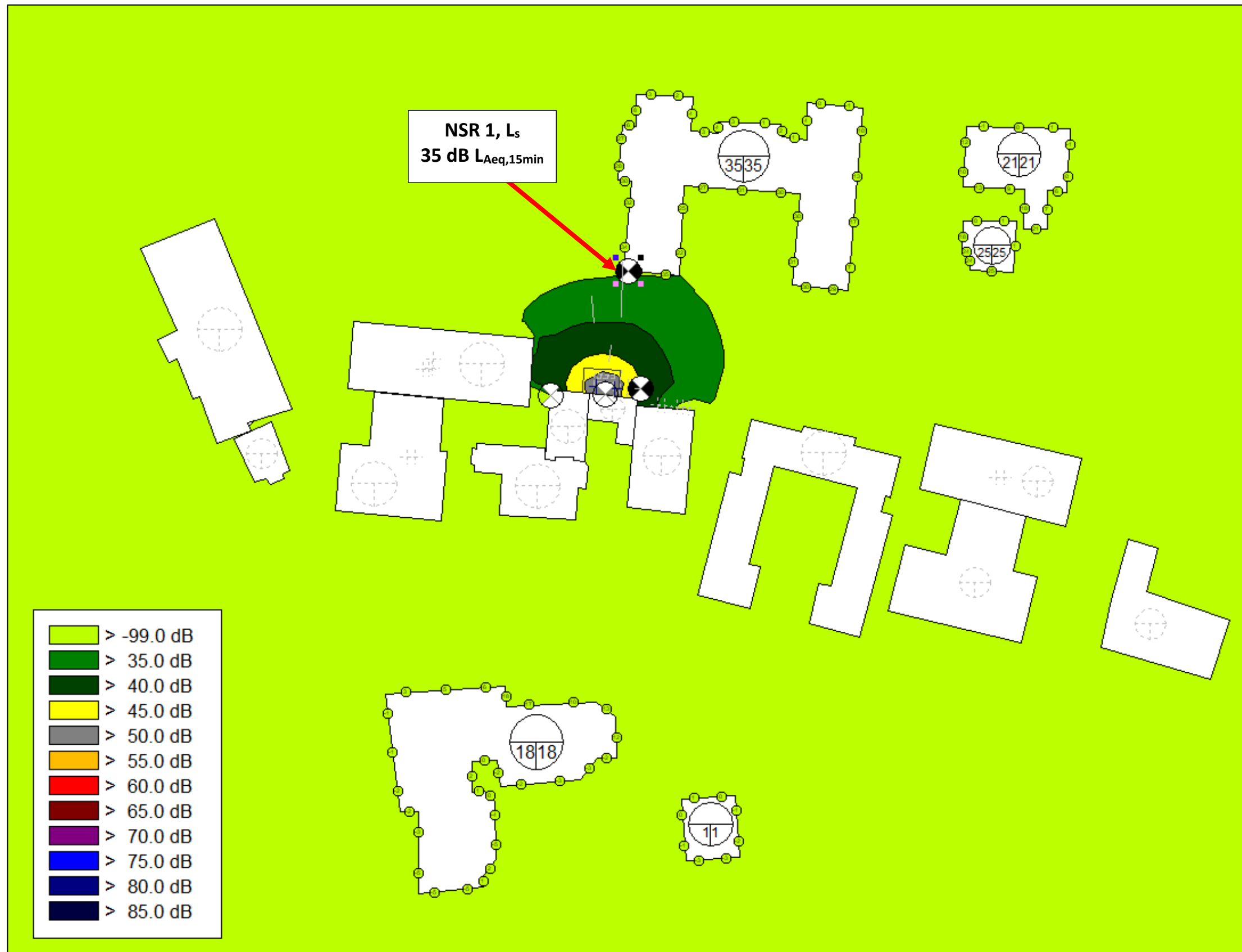
Figure 7: Sound contours at 4 m, showing the calculated specific sound level during the night-time, L_{Aeq, 15 min} based on current proposals
