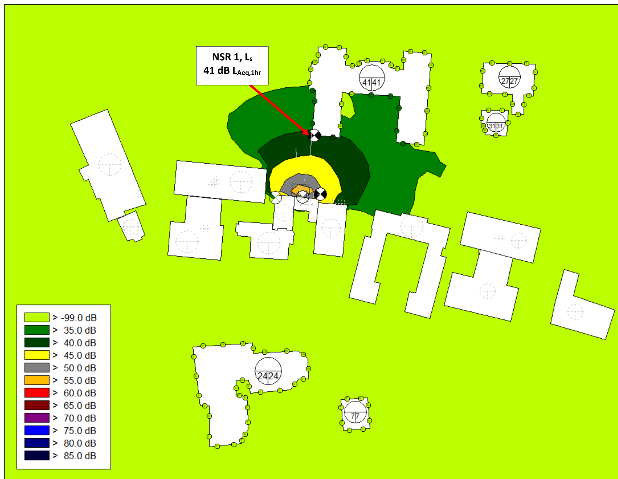
Figure 6: Sound contours at 4 m, showing the calculated specific sound level during the daytime, L Aeq 1 hr based on current proposals
