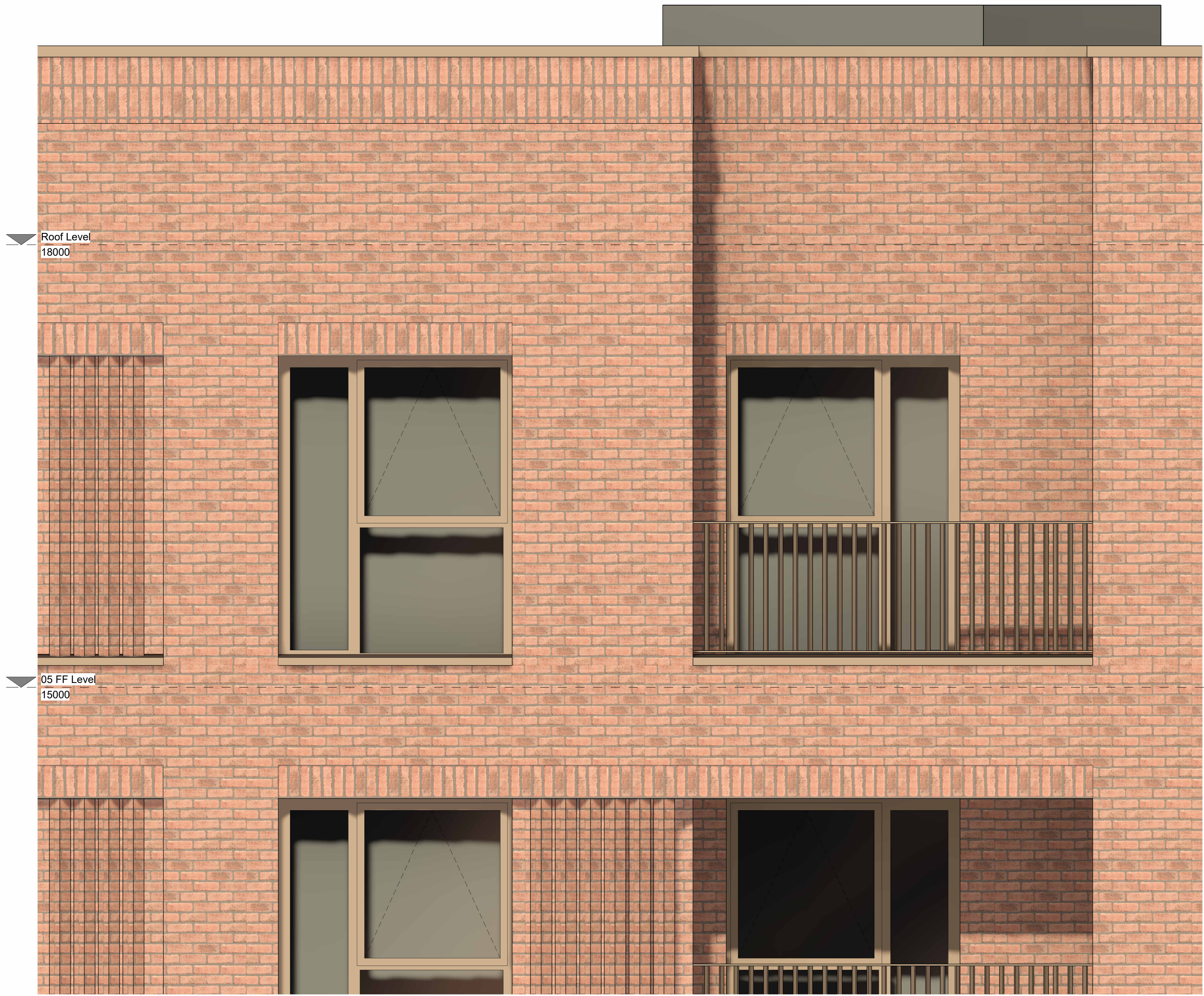
3 Recessed Balcony (East) Bay Study Elevation 1 : 20
