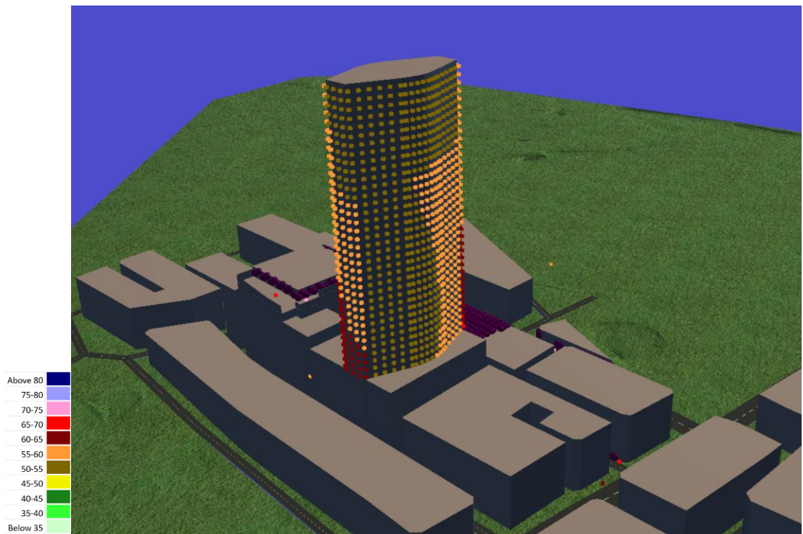
Proposed Site (looking southeast) showing incident entertainment noise levels, dB L_{Aeq,5min}
