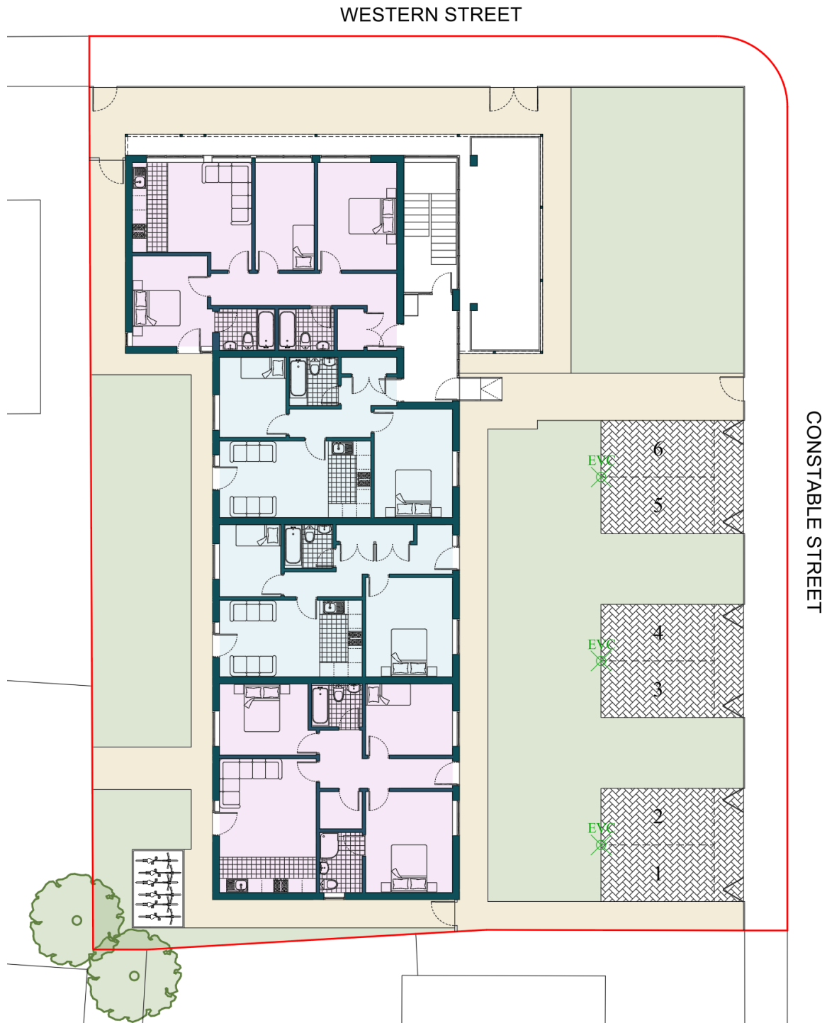
Diagram A – Proposed Site plan indicating Electric Vehicle Charging Points (Diagram not to Scale)
