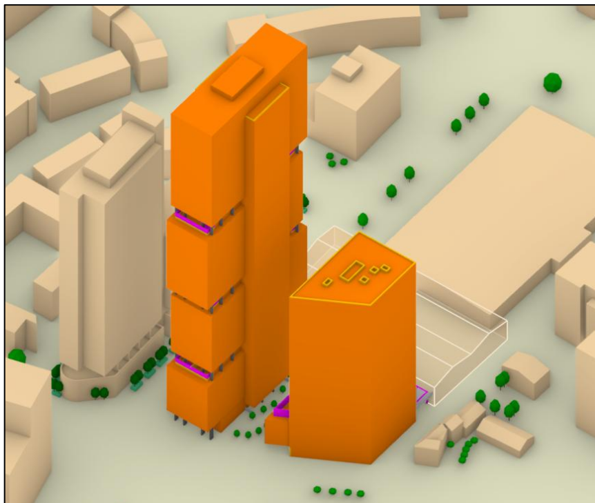
Figure C.2 – Digital model for CFD analysis
