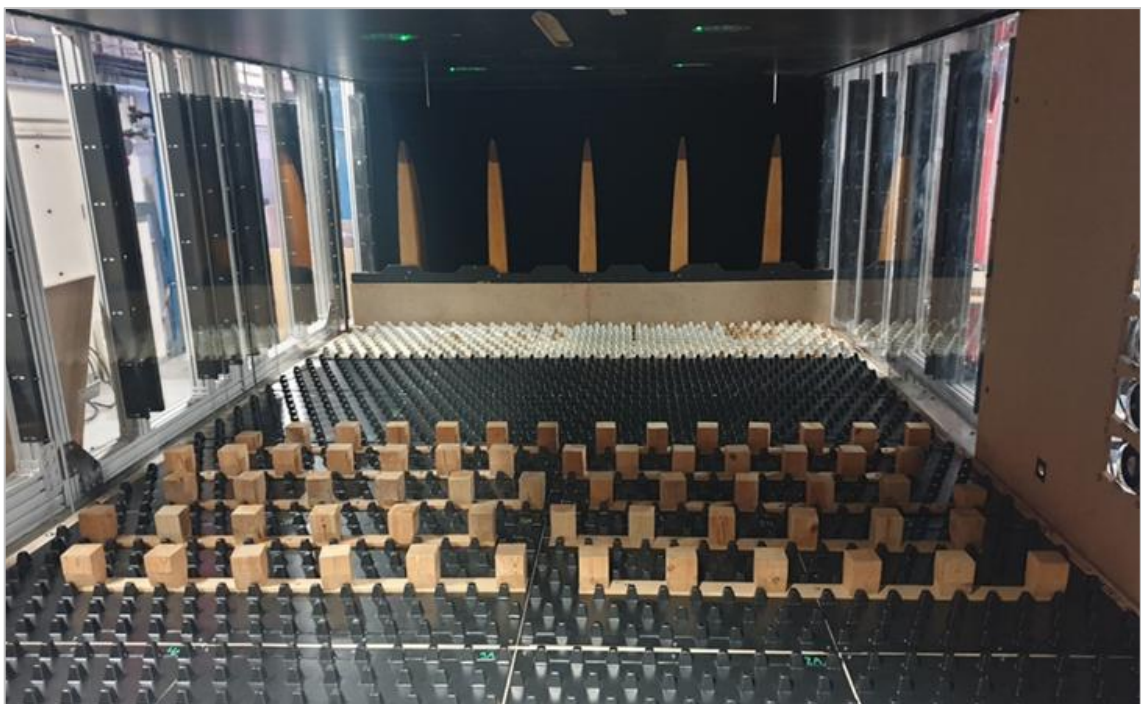
Figure A.1 - Boundary layer creation, Imperial College boundary layer wind tunnel, London.
