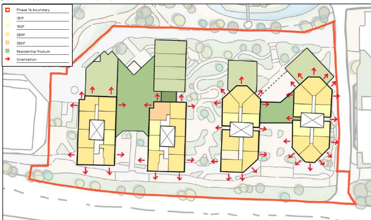
Figure 4.9 – Upper Floor Indicative Layout (ShedKM, 2024)
