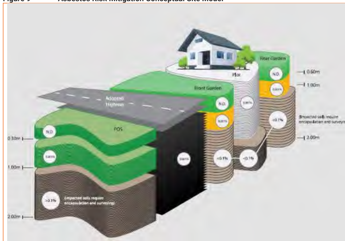
Figure 9 Asbestos Risk Mitigation Conceptual Site Model
