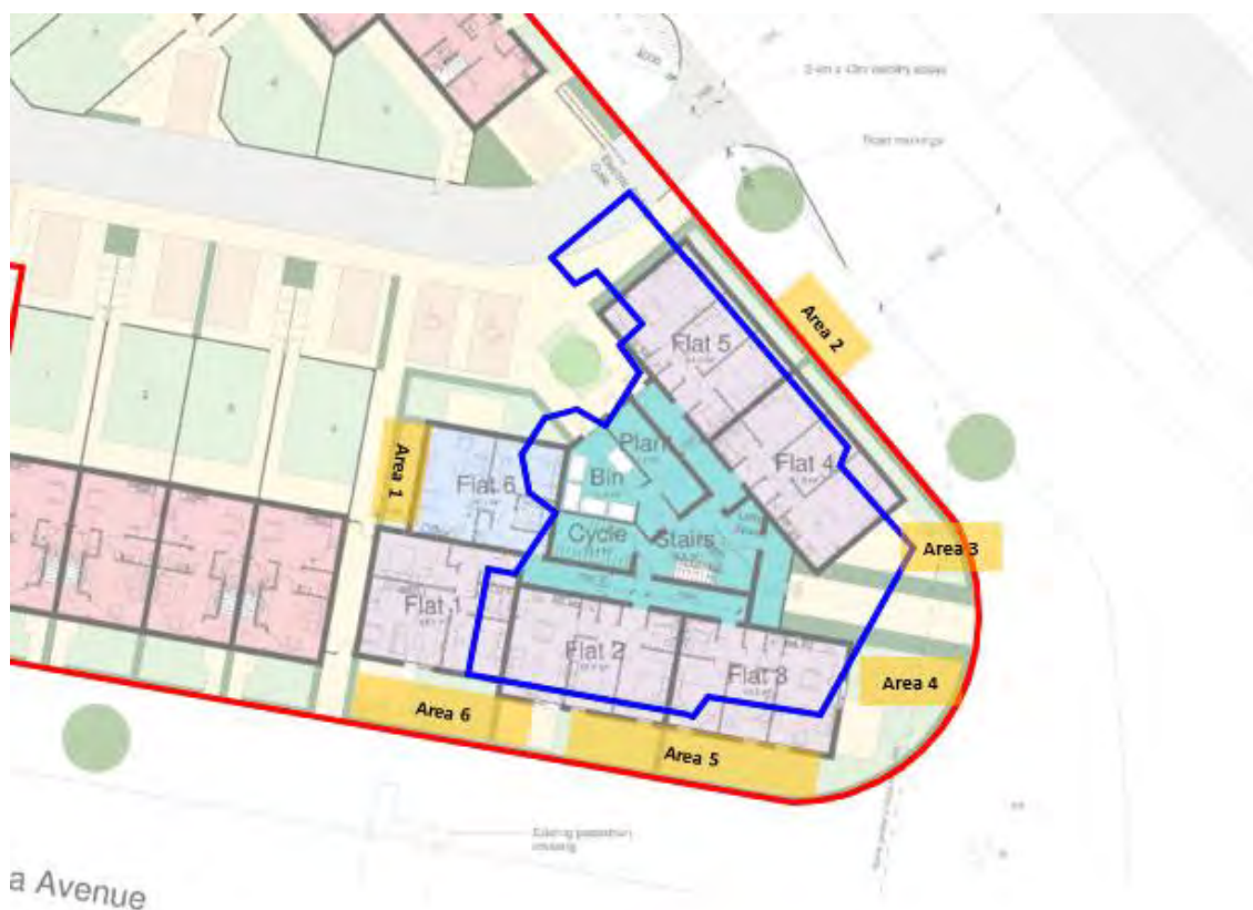
Plate 4-1: Capping layer inspection areas in apartment block soft landscaping.
