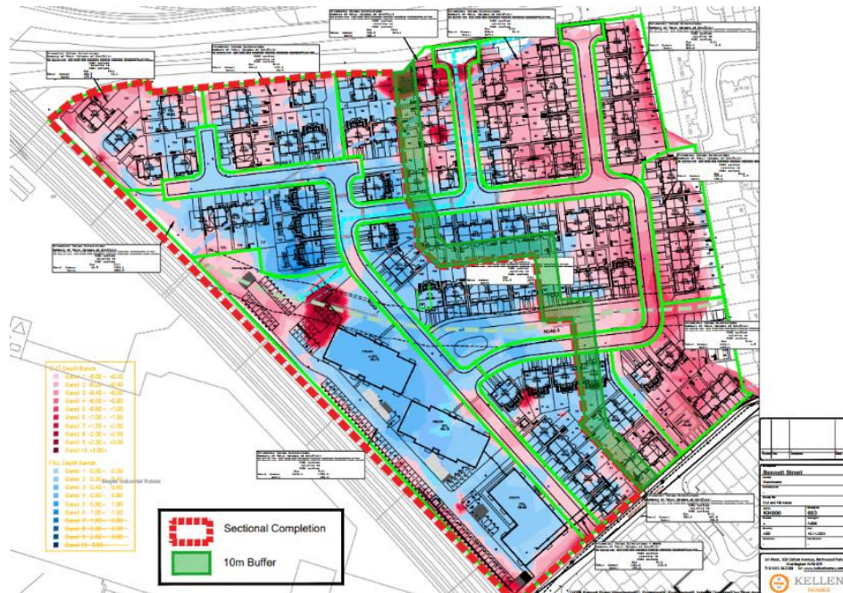
FIGURE 4.5 KELLEN HOMES CUT AND FILL SITE MODEL
