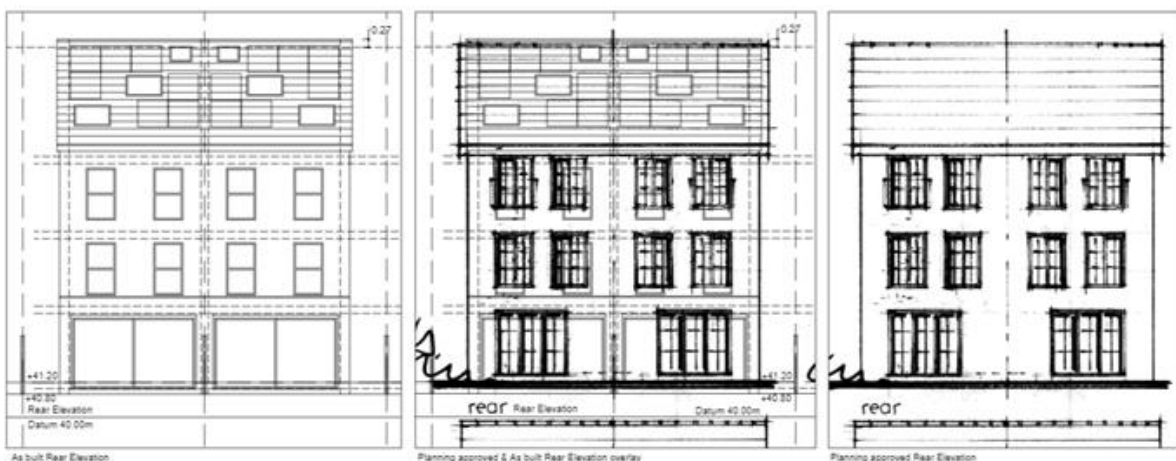
Fig.4 – Constructed and previously approved rear elevation
