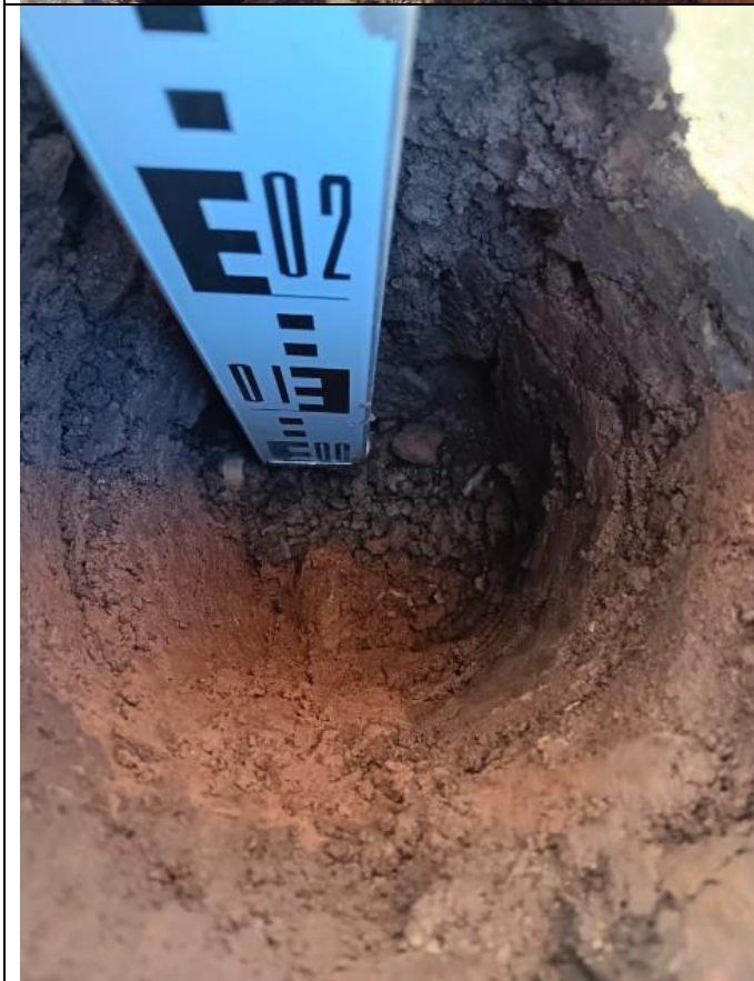
Photograph 9: View showing pea gravel in base of trial pit (area 3).
