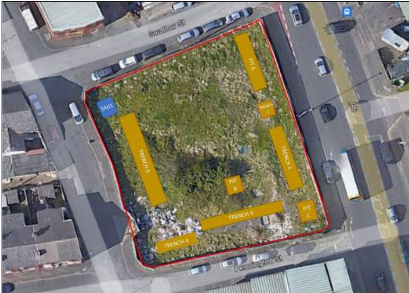
Figure 4: Exploratory Hole Location Plan (Trenching SI)
