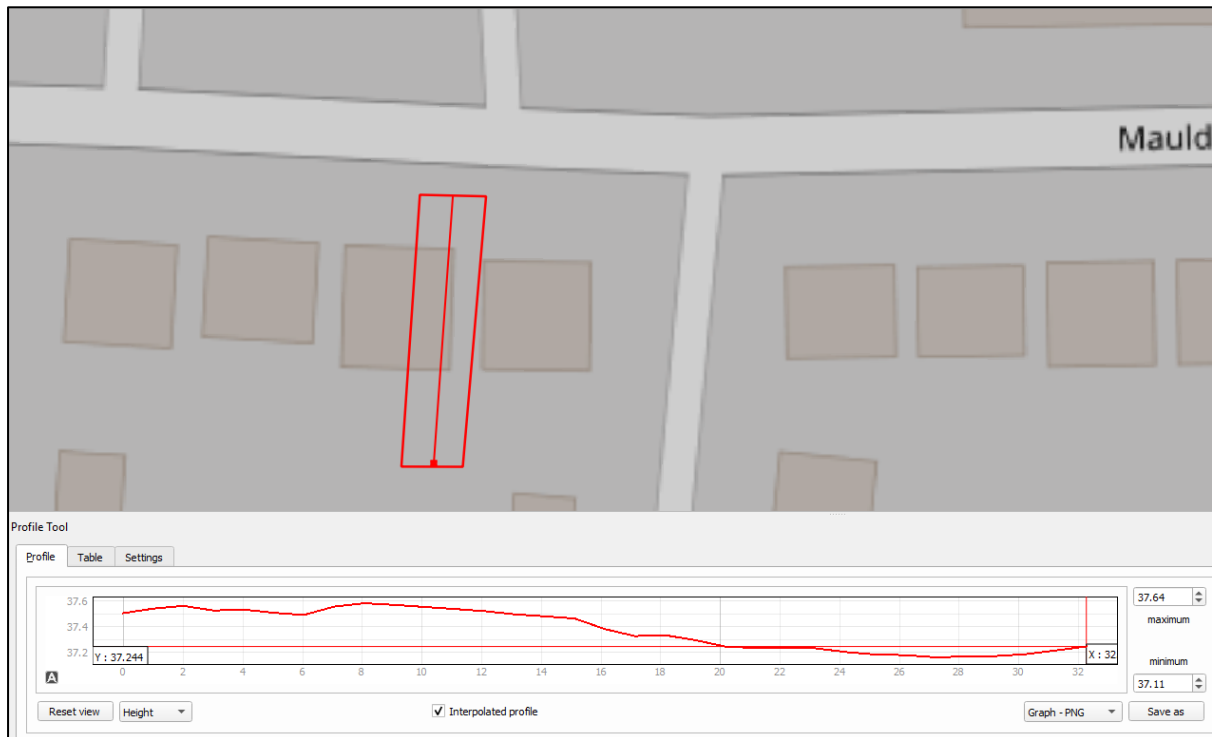
Image 1: An image showing the LiDAR undulation from north to south for 70 Mauldeth Road.
