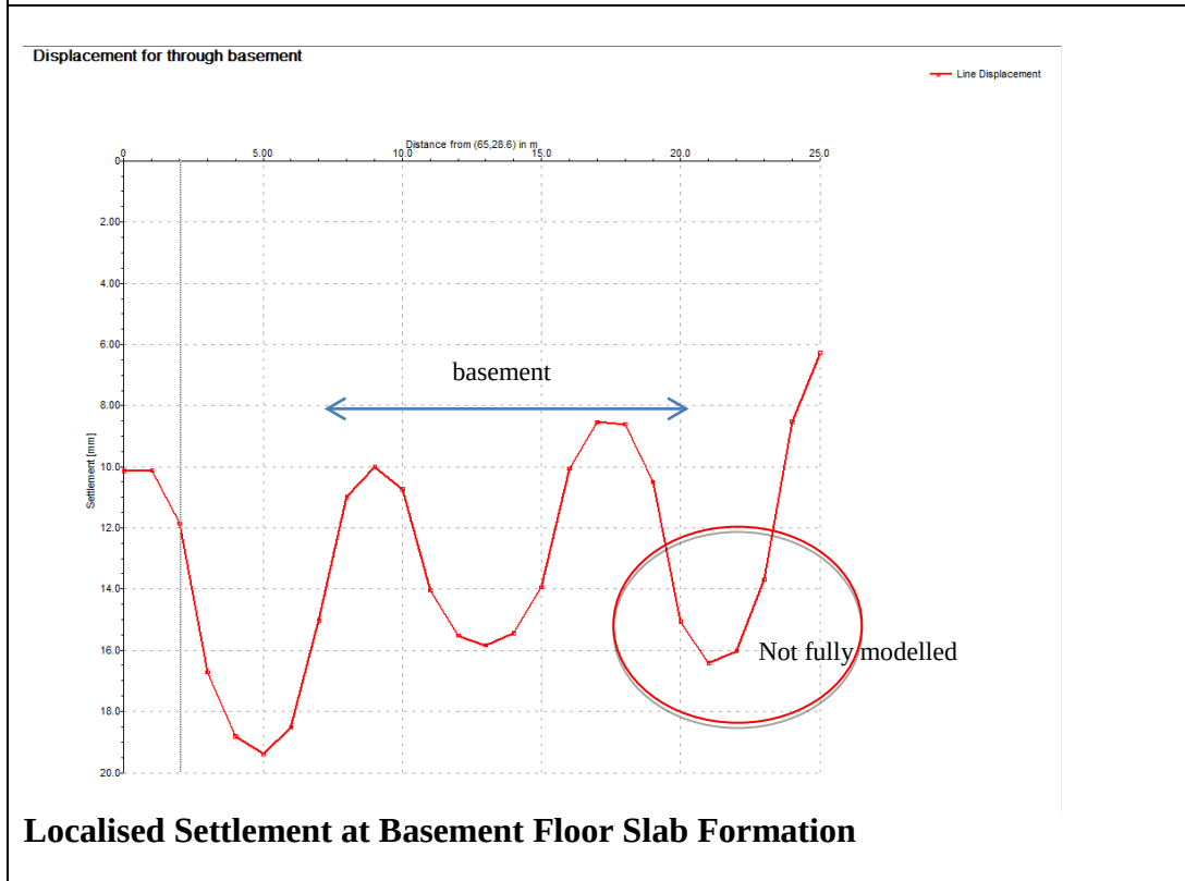
Figure 22 Run 2 Academy Building Settlement –case: pool full, DL + ave. LL for core pads
