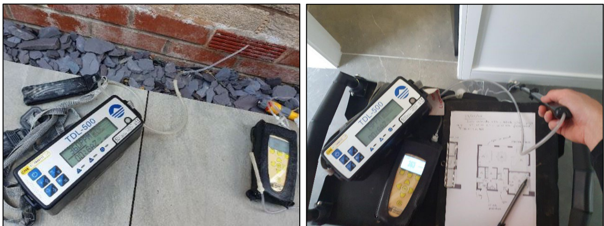
Figure 1 Selected GGS site photographs taken during the high-resolution gas sweep surveys undertaken at the site. Left: Photograph of measurements taken from a selected air brick via semi rigid sample tubing. Right: Photograph taken during the internal gas sweep survey.
