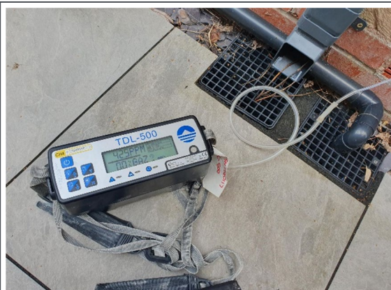
5. Methane measurement of an air brick.
