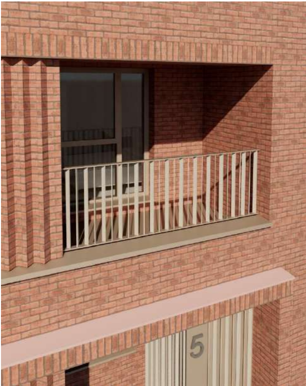
Balcony and balustrade detail
