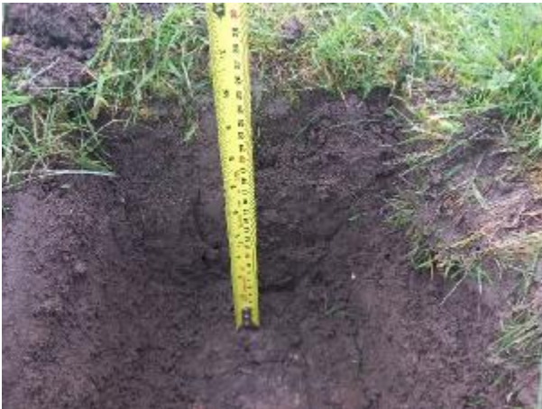
Photo 19: Excavated test pit.
