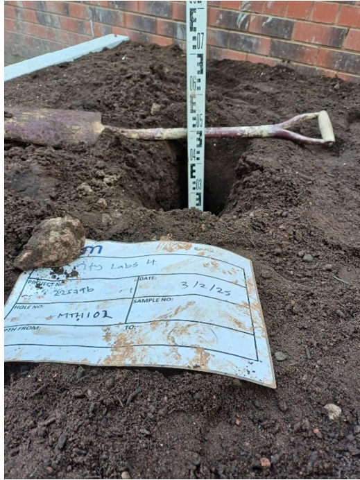
Plate 5: Depth check at MTH102, displaying a depth of 480 mm.
