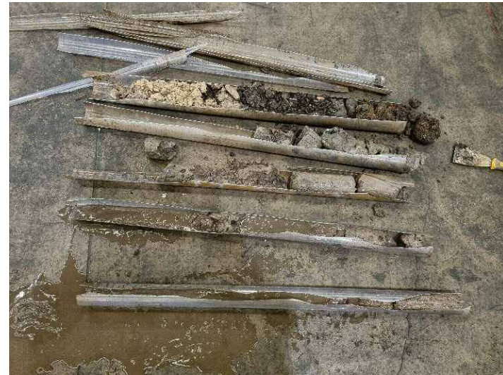
Photograph 12 – Core recovery of borehole WS07.
