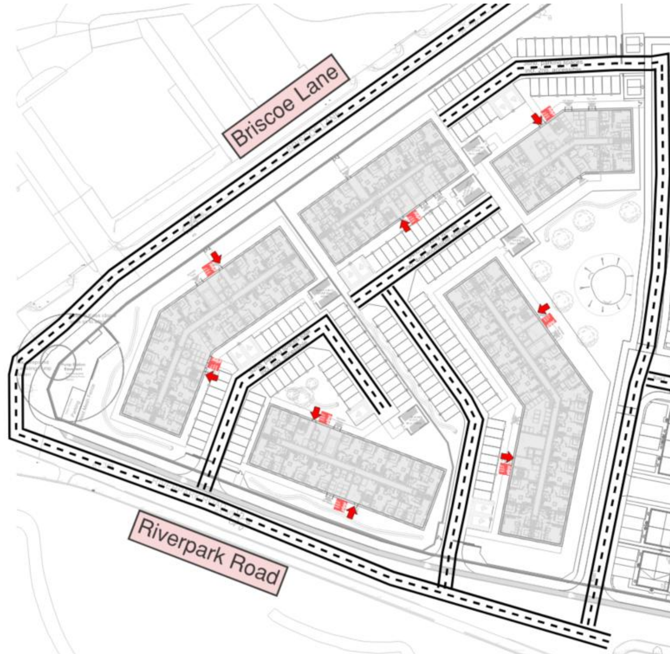
Figure 2 – Fire service access
