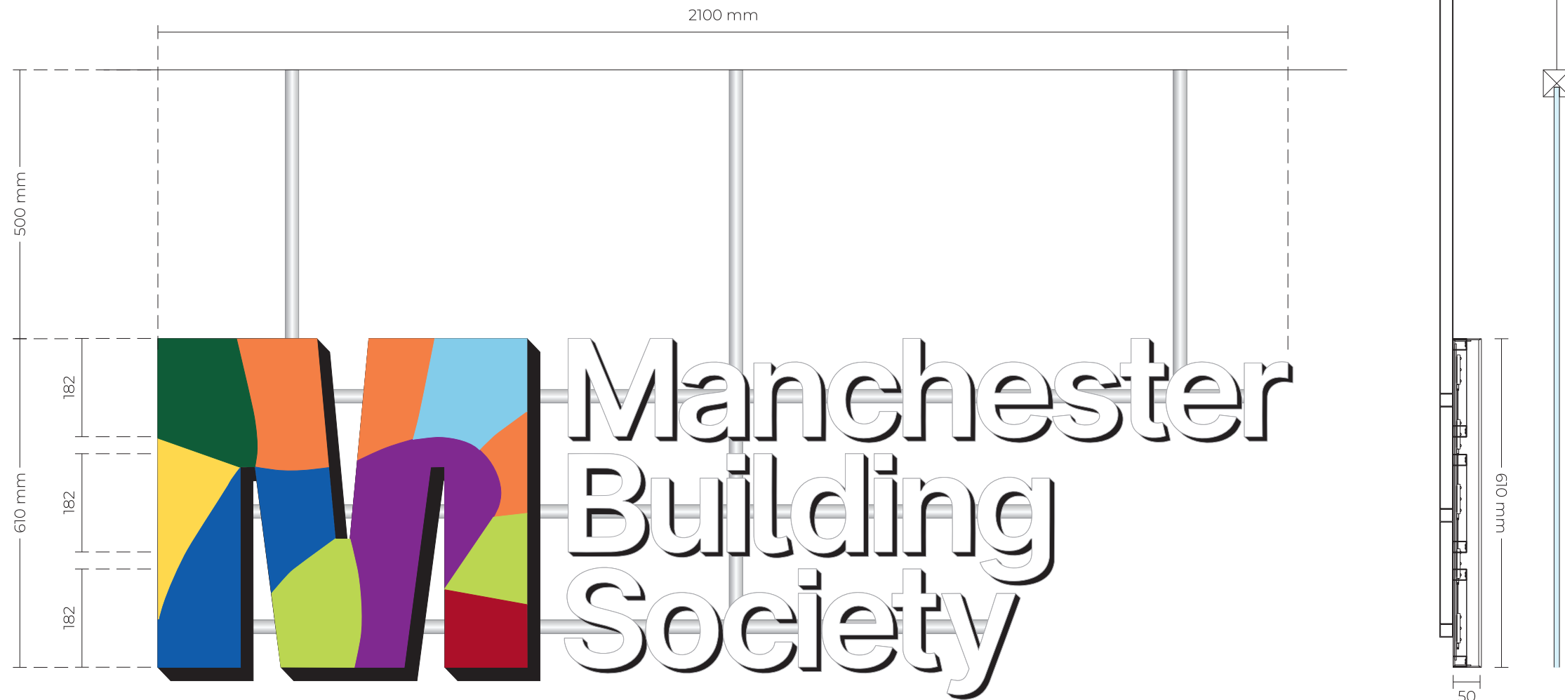
3no. Suspended Window Signs Scale 1:10 @ A3
