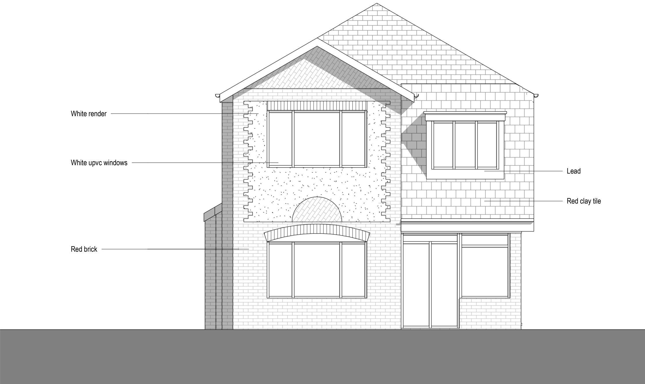
EXISTING ELEVATIONS - NORTH WEST 1 : 50
