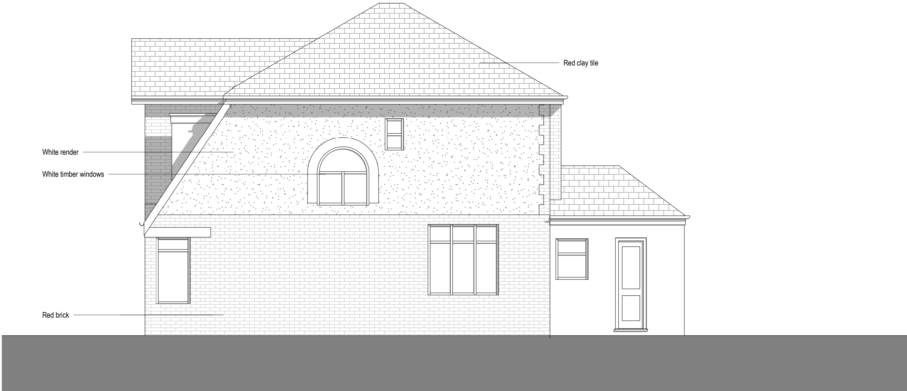
EXISTING ELEVATIONS - SOUTH WEST 1 : 50
