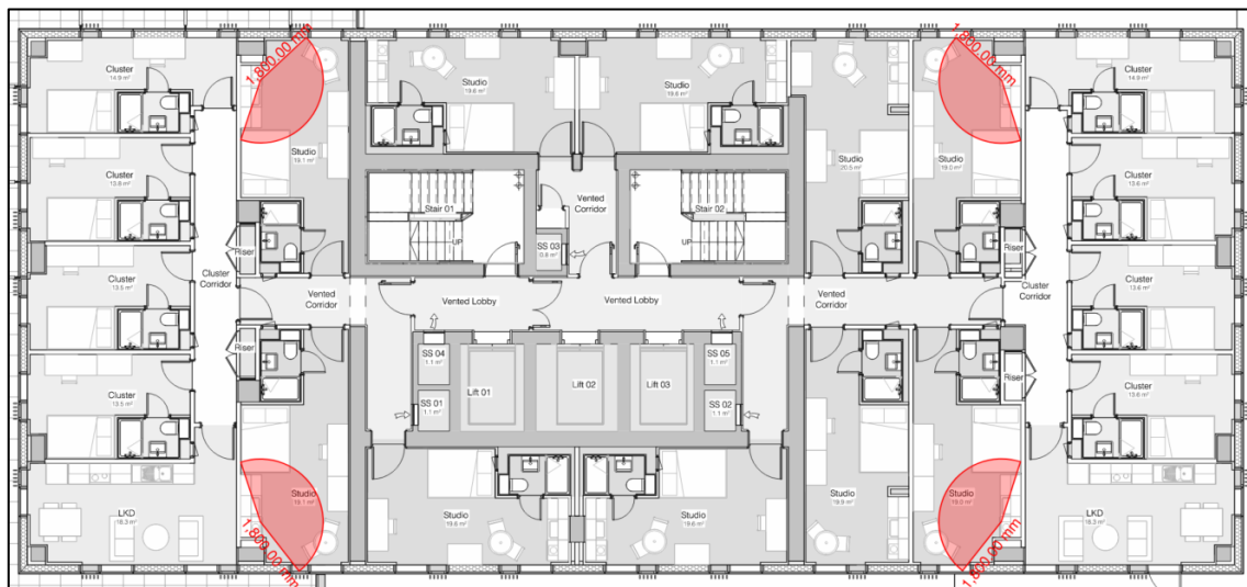
Figure 11: Sleeping Accommodation within 1.8m of the Hob Edge
