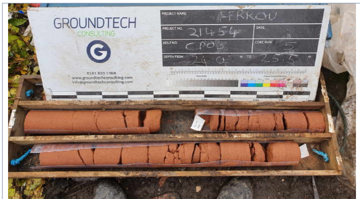
Photograph 21 – CP03 Rotary core run 5.
