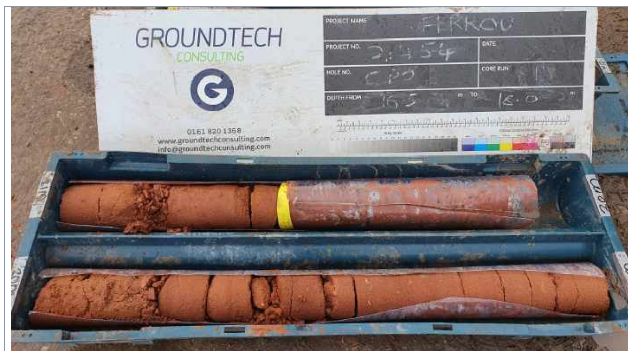
Photograph 24 – CP04 Rotary core run 1
