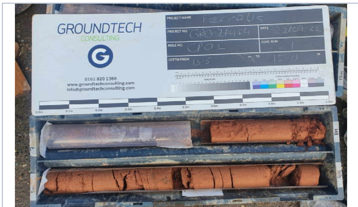
Photograph 11 – CP02 Rotary core run 1.
