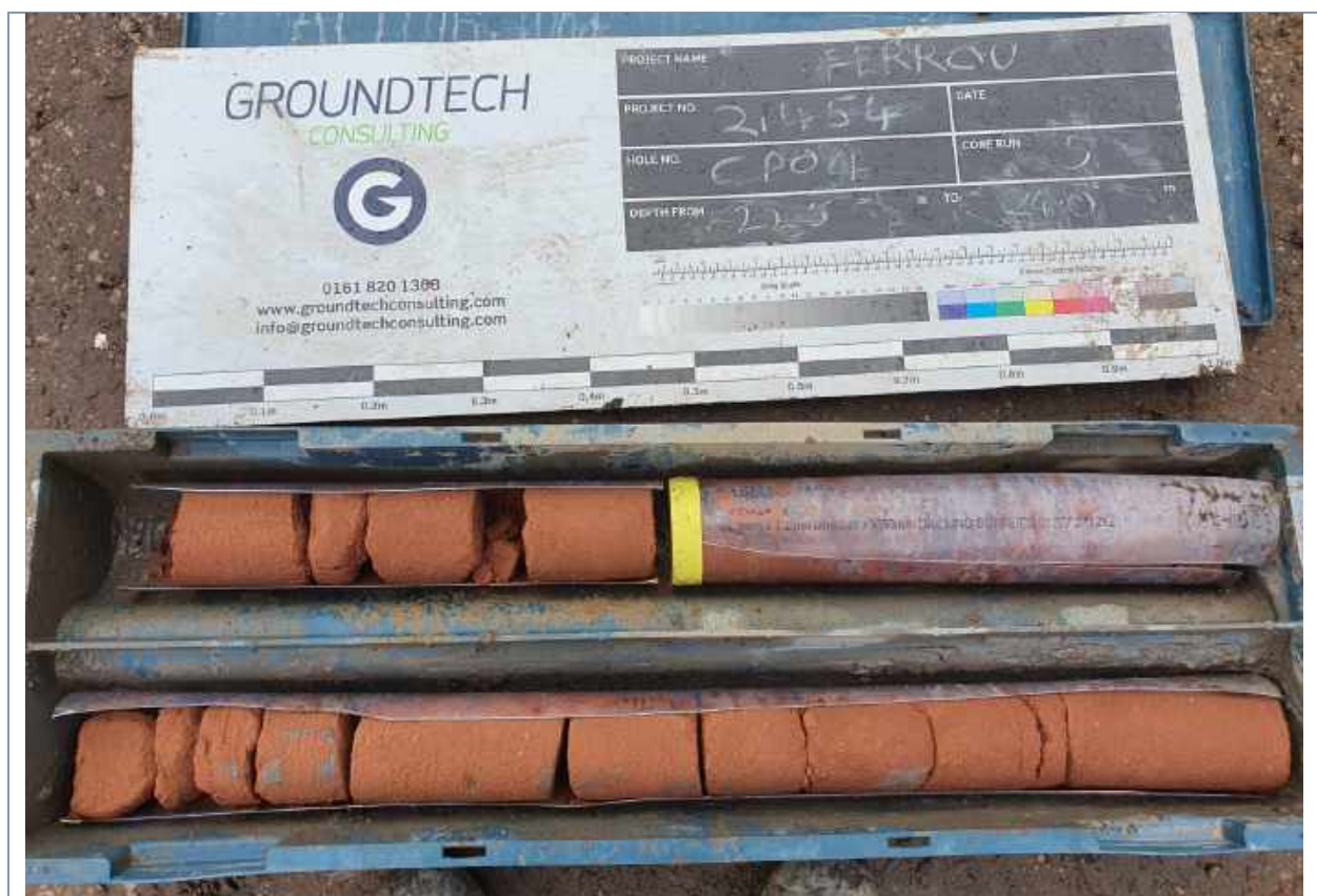
Photograph 28 – CP04 Rotary core run 5
