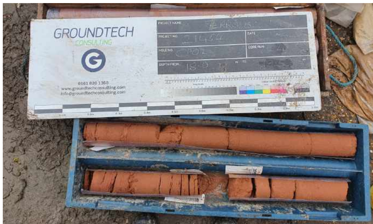
Photograph 14 – CP02 Rotary core run 4.
