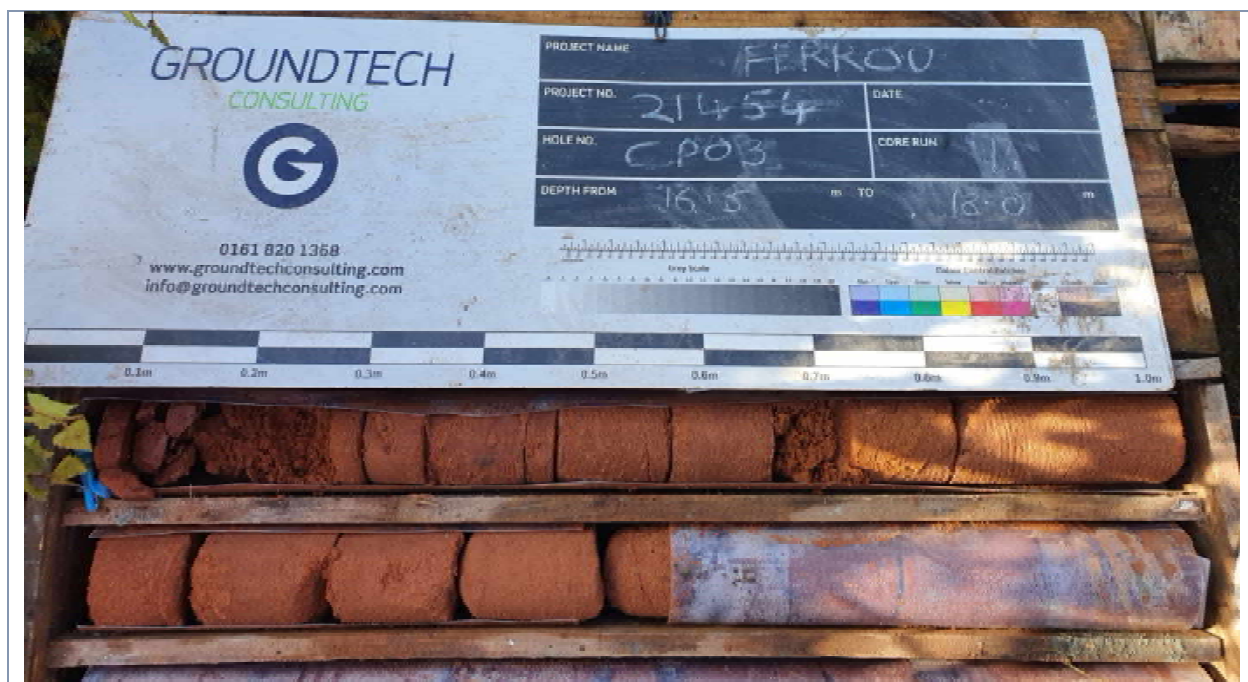
Photograph 17 – CP03 Rotary core run 1.
