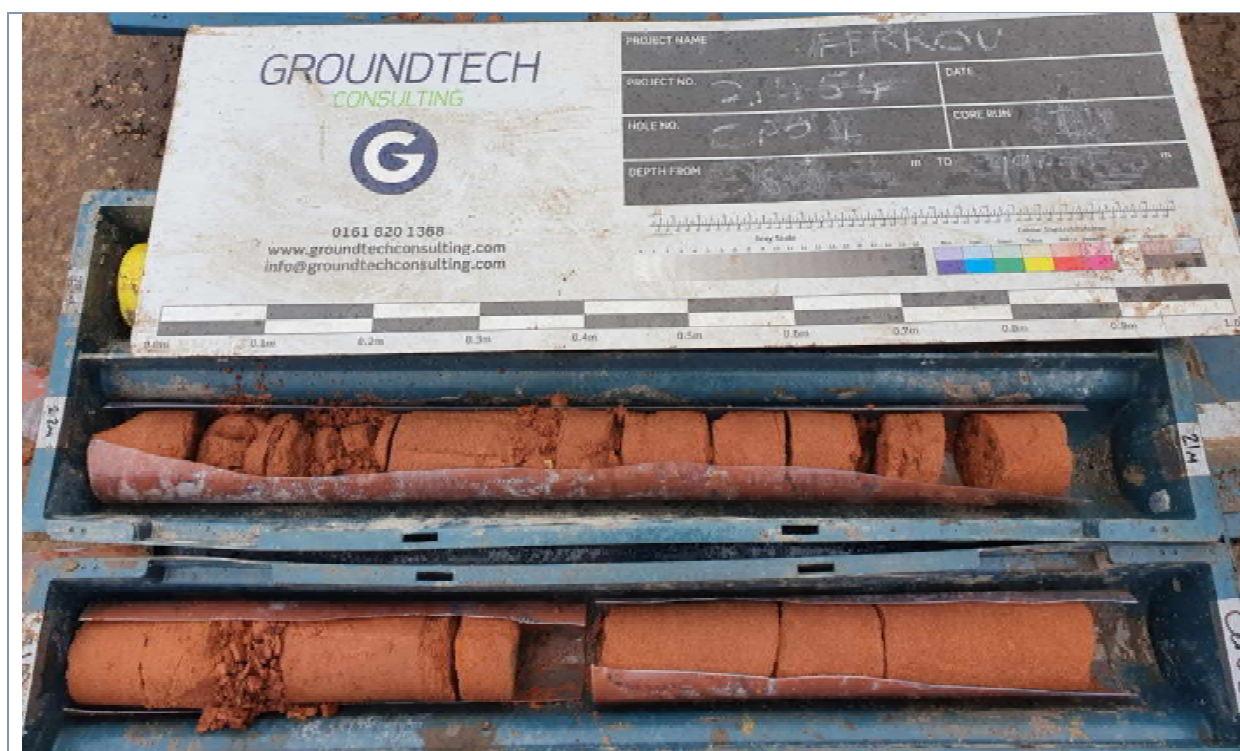
Photograph 25 – CP04 Rotary core run 2.
