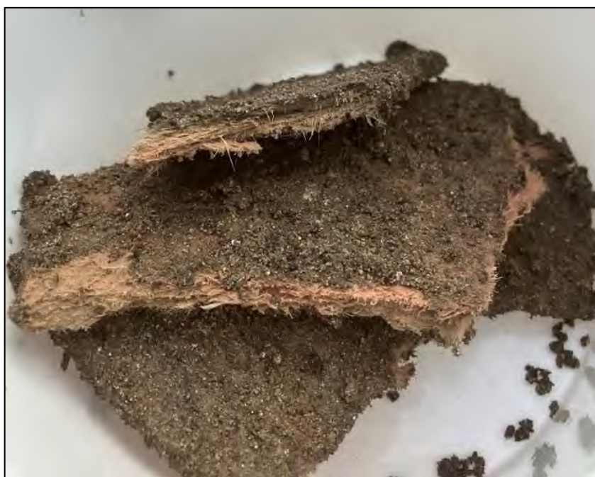
Figure 7-A: Suspected ACM observed within Made Ground deposits from TP01
