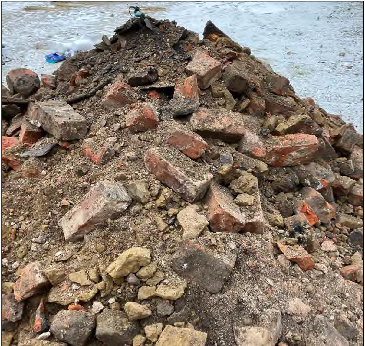
Figure 5-A: Made Ground deposits encountered in TP02
