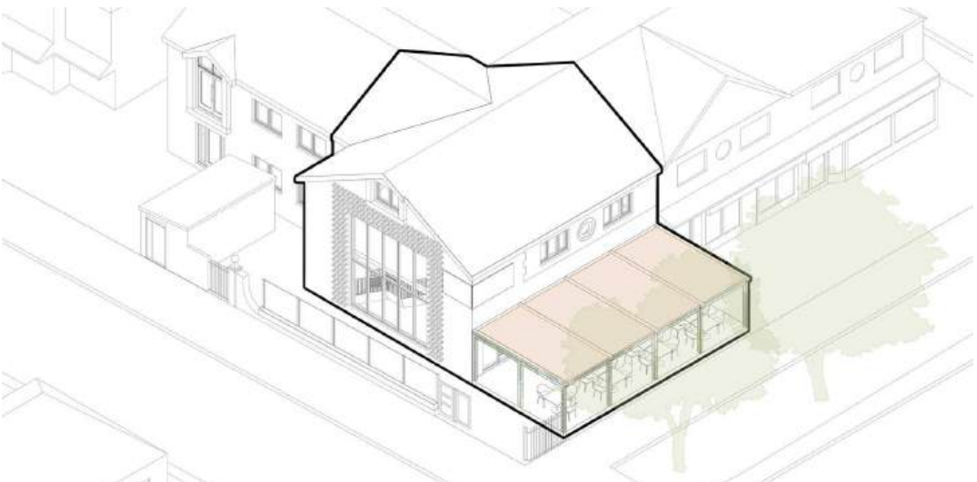
Retractable Roof Fabric Replaced with Lighter Colour: Reducing its visual dominance while improving solar reflectivity. Enhances thermal comfort within the restaurant and creates a more subtle and cohesive appearance.
