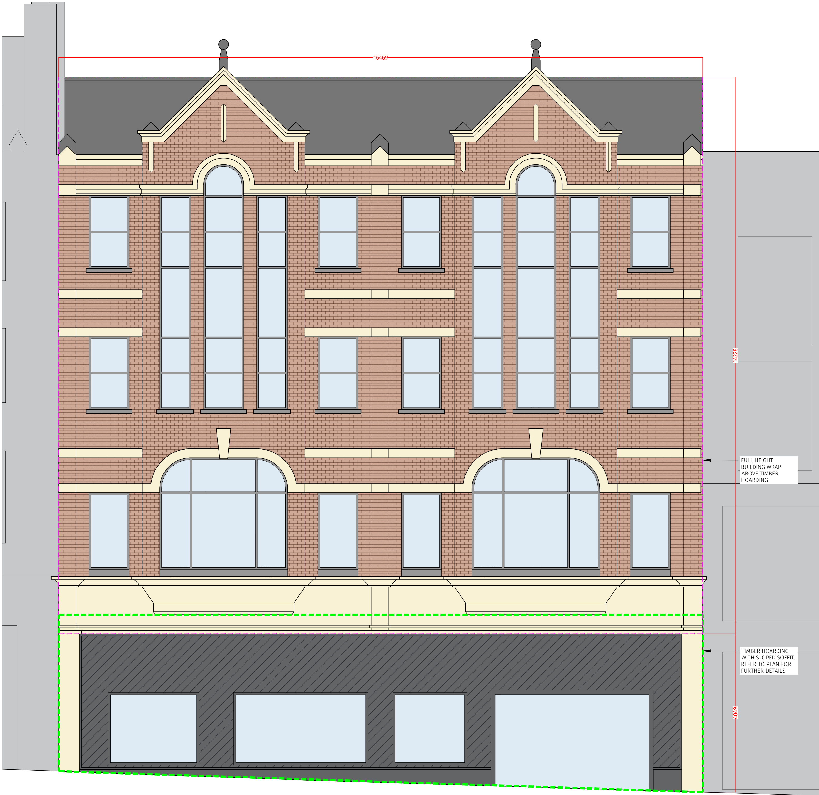
02 | Proposed Hoarding Elevation SCALE:1:50
