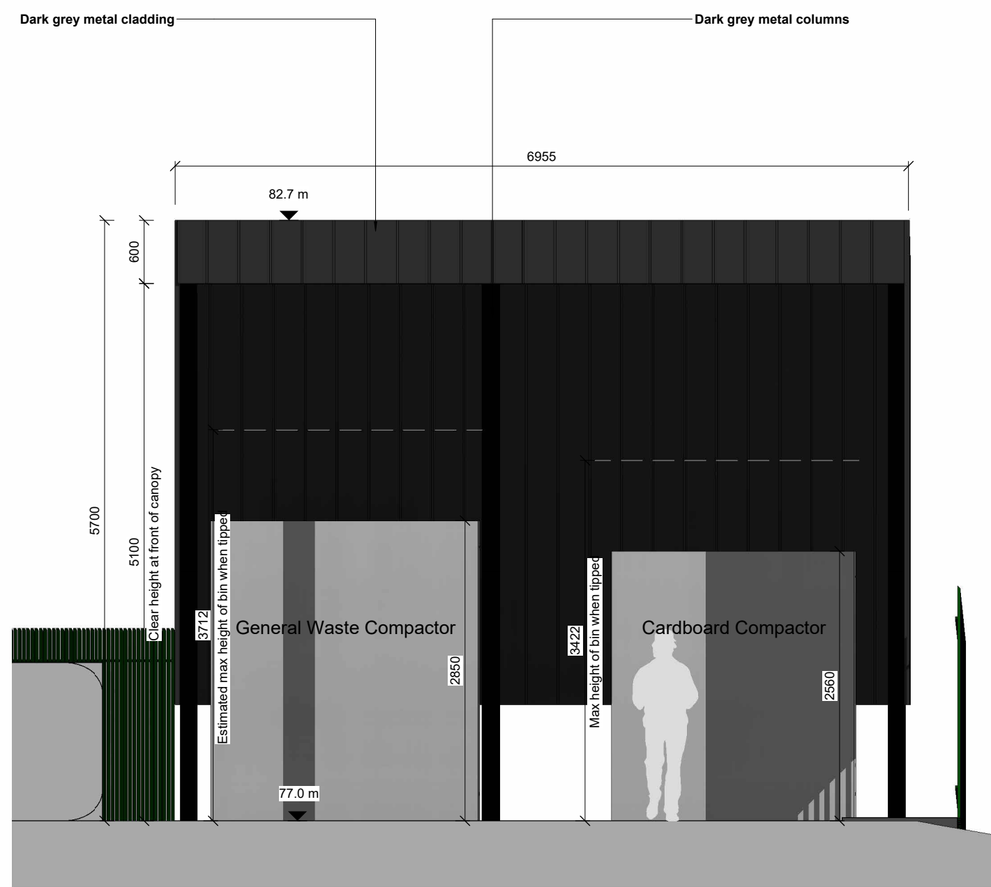
2 Compactor Canopy North Elevation 1 : 50
