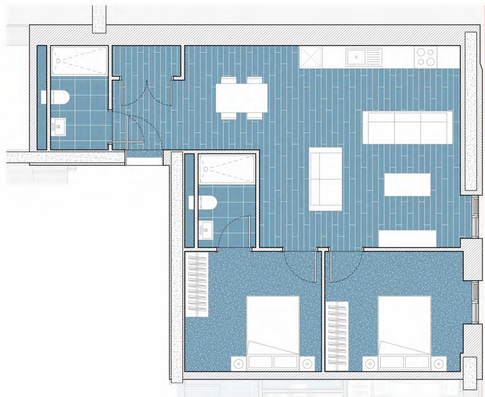
Typical 2 bed 4 person apartment. 72 sq.m. 1:100@A3
