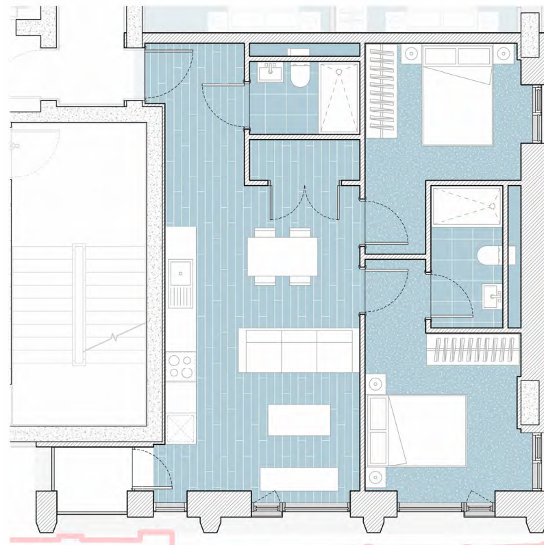
Typical 2 bed 3 person apartment with balcony. 61 sq.m. 1:100@A3
