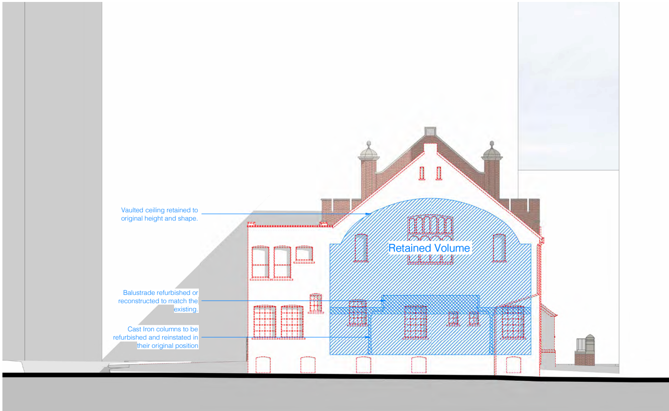
North West Elevation
