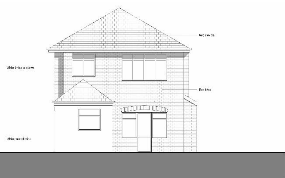
EXISTING ELEVATIONS - SOUTH EAST 1:50
