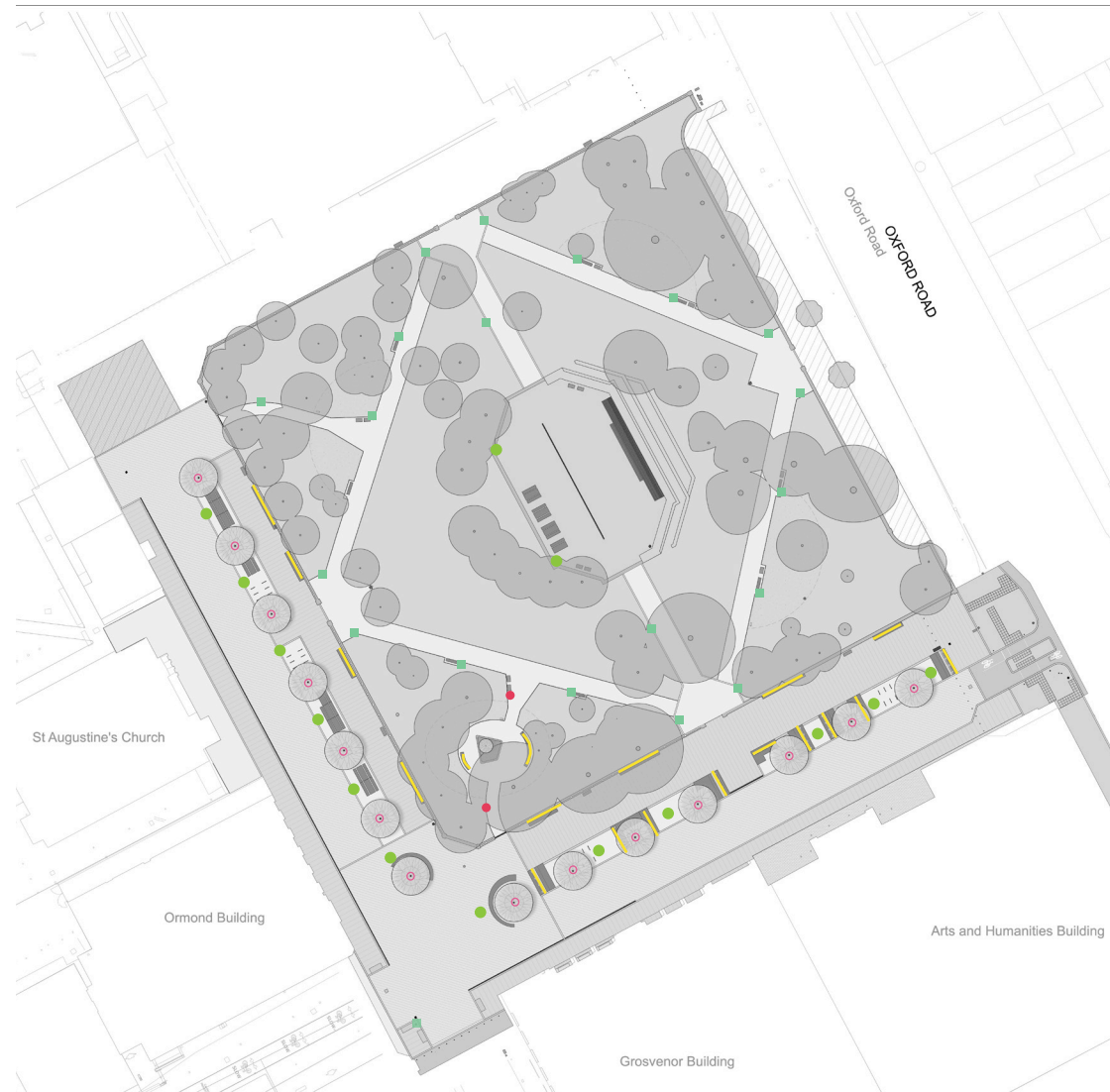
Lighting Arrangement, Phase 1A
