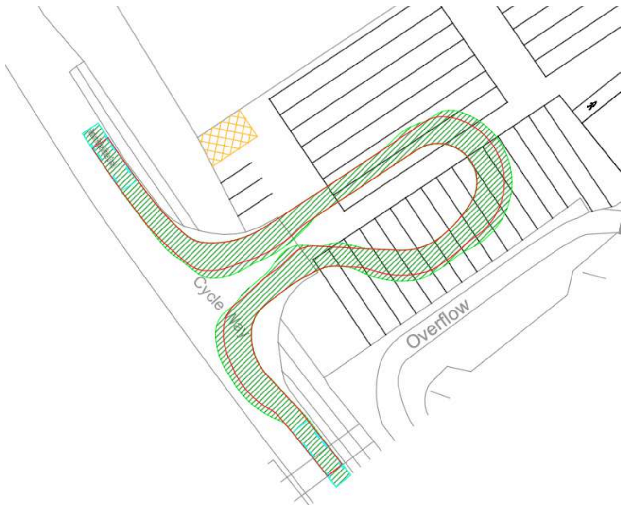
Figure 5.1 : Swept Path Analysis – 11.2 Refuse Collection Vehicle
