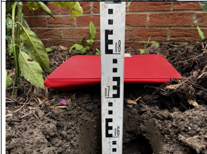
Photograph 4: Evidence of suitably chemically validated topsoil with a minimum of 150mm growing medium in front garden area (Plot 5) over natural strata.
