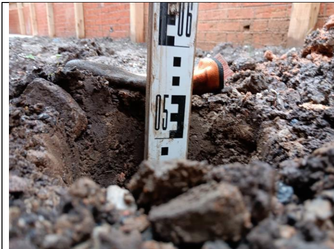
Photograph 2: Evidence of suitably chemically validated topsoil with a minimum of 150mm growing medium in rear garden areas (Plot 5) over natural strata.
