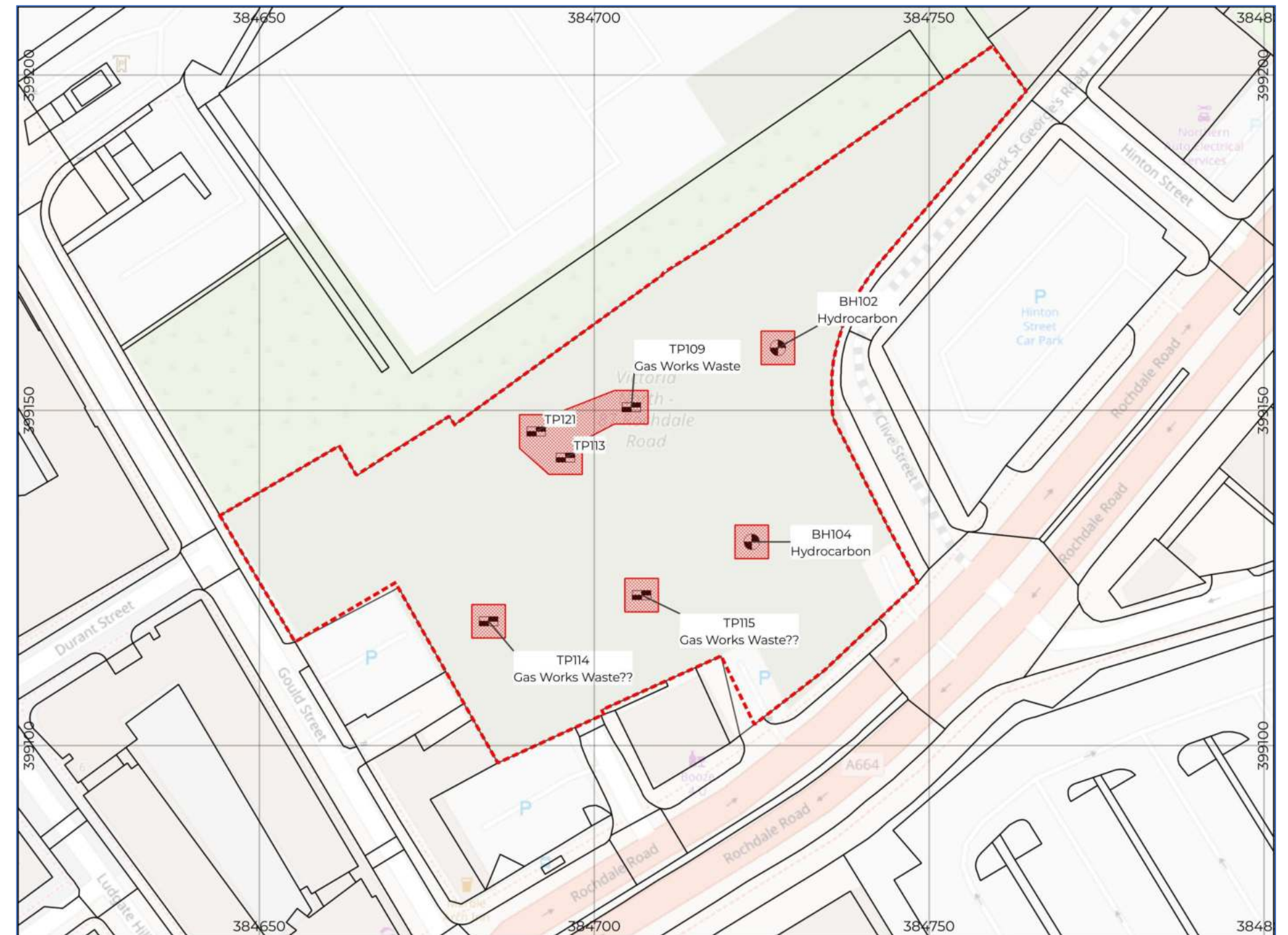
Figure 7 Hotspot Removal Excavations
